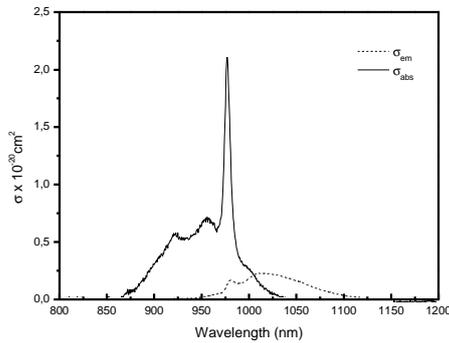
Figure 1. Absorption and emission cross-sections spectra for the heavy metal oxide glass with 0.5mol% of  $\text{Yb}_2\text{O}_3$ .
