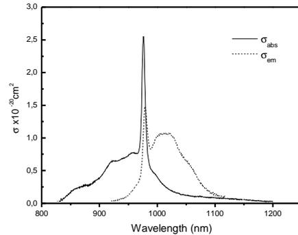
Figure 2. Absorption and emission cross-sections spectra for the lead fluoroborate glass with 0.5mol% of  $\text{Yb}_2\text{O}_3$ .
