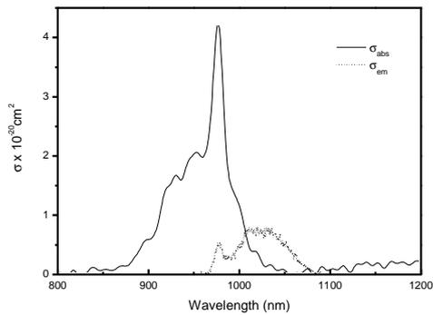
Figure 3. Absorption and emission cross-sections spectra for the niobium tellurite glass with 5mol% of  $\text{Yb}_2\text{O}_3$
